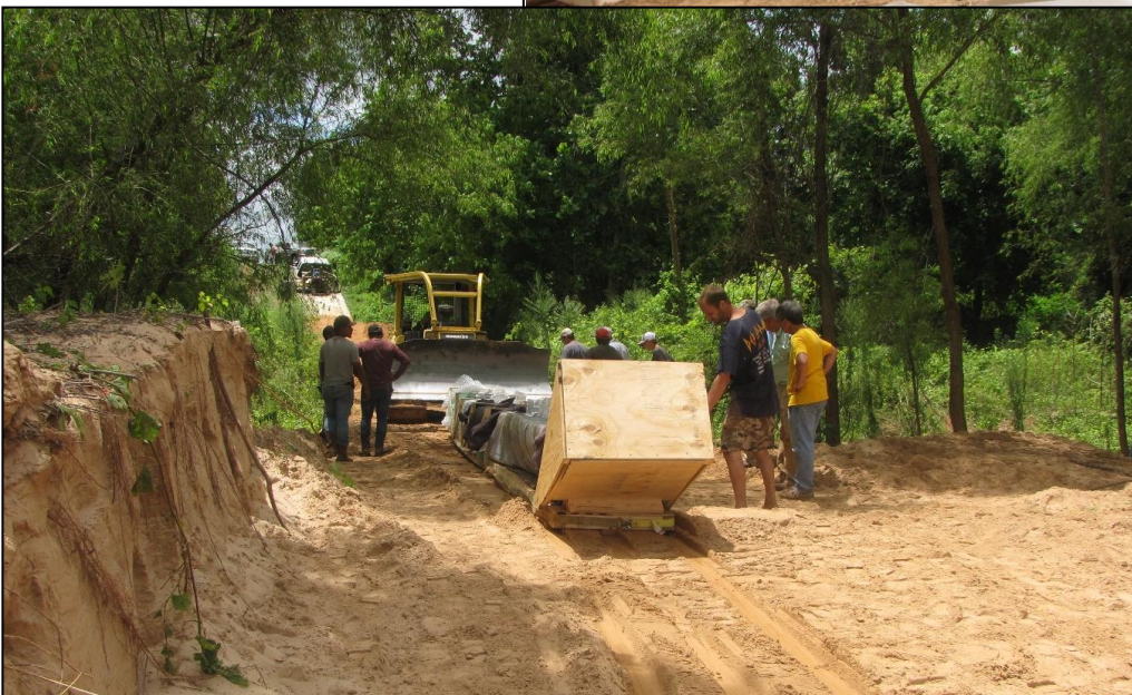
Figure 5. Bulldozer dragging platform toward the waiting flatbed trailer in background.
